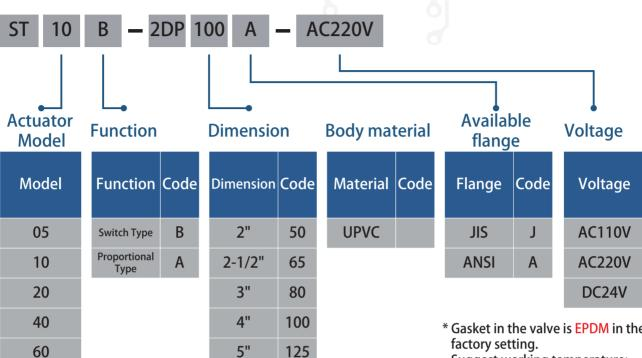
\* Actuator Proportional type Input / Output signal 4 - 20 mA.DC in factory setting.
