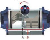
Compressed air input by **A Port**, make the piston and output shaft turn counterclockwise. Open the valve. Expel the air in the piston by **B port**.
