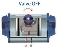
Compressed air input by **B Port**, make the piston and output shaft turn clockwise. Close the valve. Expel the air in the piston by **A port**.
